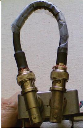
Completed Polarity Switching Preamp, with 70CM Phasing Line
