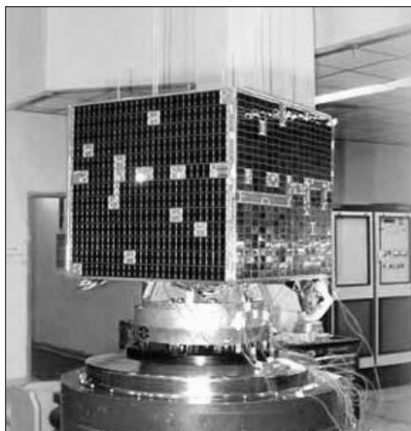
Photo 1: VO-52 sits atop its carrying structure just prior to integration into its PSLV-6 launch vehicle. (Courtesy: AMSAT-India)
