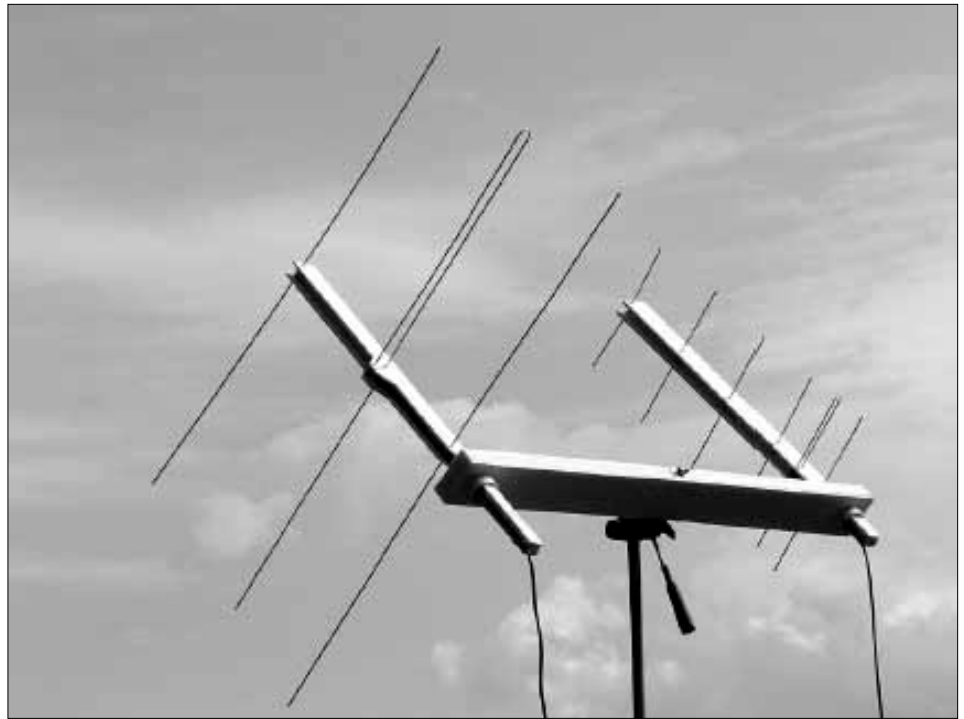
Satellite antennas don't need to be fancy to be effective. Here, a pair of vertically polarized, home brew Yagi antennas made from bits of wire and wood are mounted on a wooden cross boom. (Courtesy: AMSAT)
