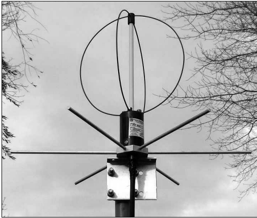
This photo shows a view of the author's 70cm, M2 Eggbeater antenna. Note the ground radials mounted underneath the phasing coil. (Courtesy: KB1SF)
