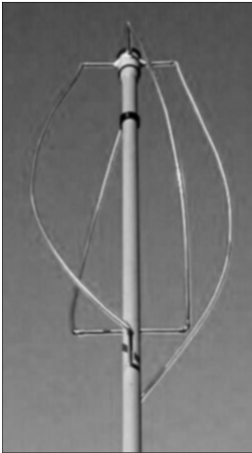
The Quadrafil Helix antenna is a relatively easy to build, omnidirectional antenna that can be optimized for both Amateur Radio and weather satellite work. (Courtesy: Bob Cash, N8IMO)
