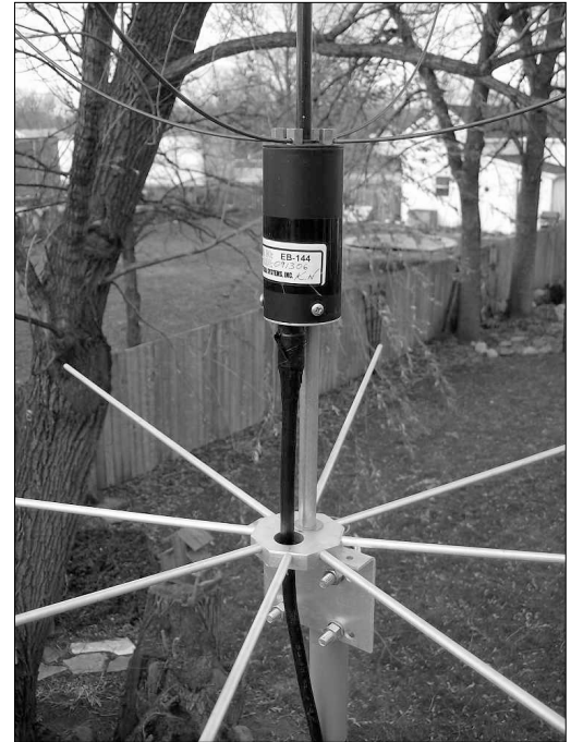
Here's a partial view of the phasing coil and ground plane of the author's 2 m, M2 Eggbeater antenna. Note that the ground plane radials are offset by about 1/2 wavelength (10.5 inches) from the top of the phasing coil and driven elements. (Courtesy: KB1SF)
