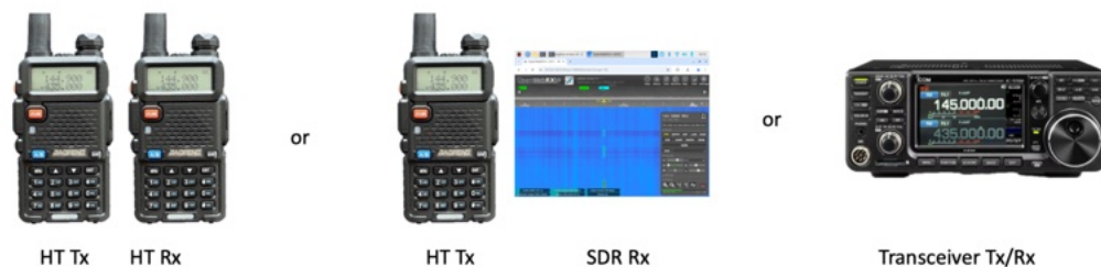
Figure 4. Radio Options for the Cross Band Repeater Mode: Two HTs, One HT and one SDR, or One Full Duplex Transceiver
