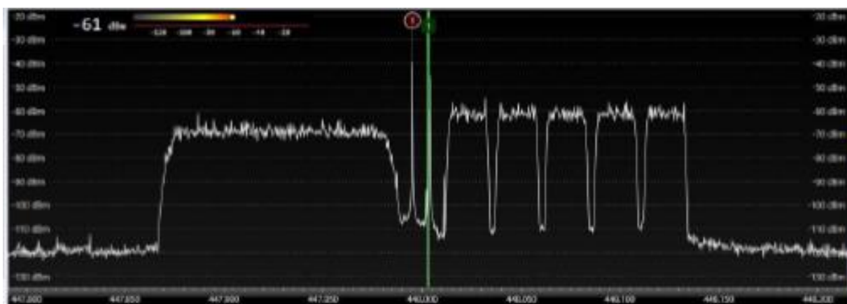
FIGURE 7: Example SDR Transponder Communication Mode Spectrum
