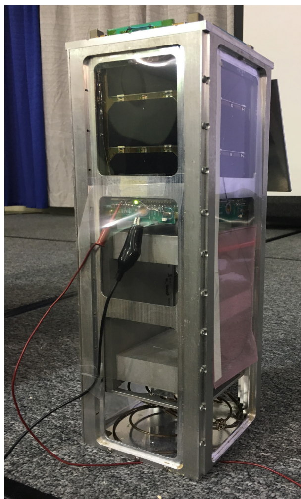
Bob demonstrated a functioning digital satellite model transmitting on 145.825 MHz APRS/packet to attendees [Joe Kornowski, KB6IGK, photo].
