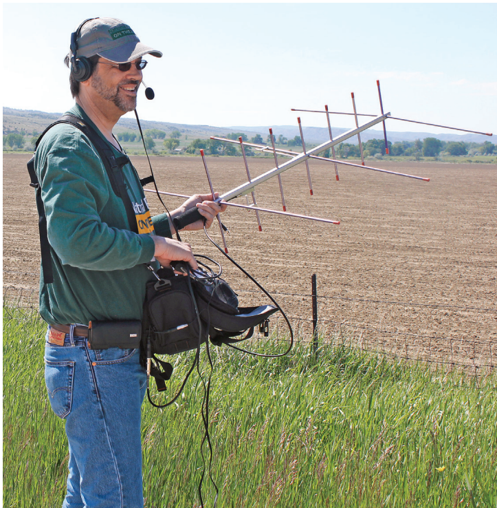
Many satellite operators use an extremely portable full-duplex station built around two Yaesu FT-817 transceivers for both FM and SSB (linear) satellites. The author used this setup when roving through Montana in May 2017. [Katie Allen, WY7YL, photo]
