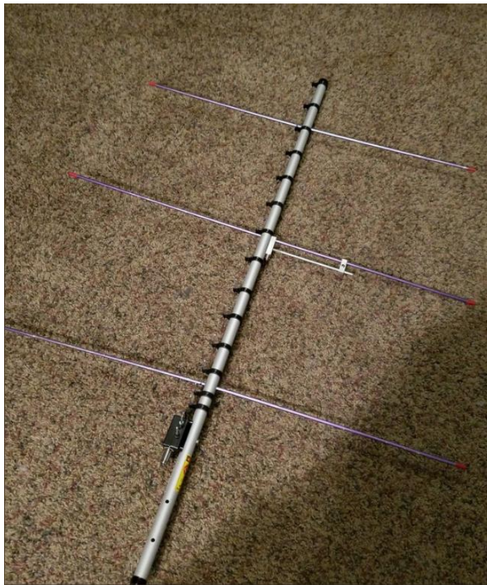
A Comet CYA-1216E Yagi modified with Arrow II 2 meter elements for portable Mode L/v operation (Photo courtesy ACORA)
