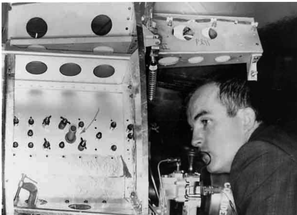
Lance Ginner, K6GSJ, looks over the carrying structure that will loft OSCAR-I to orbit on the CORONA upper stage. Note the faint arrow pointing to OSCAR-I's $1.15 Sears-Roebuck spring ejection mechanism. [Lance Ginner, K6GSJ, photo.]
