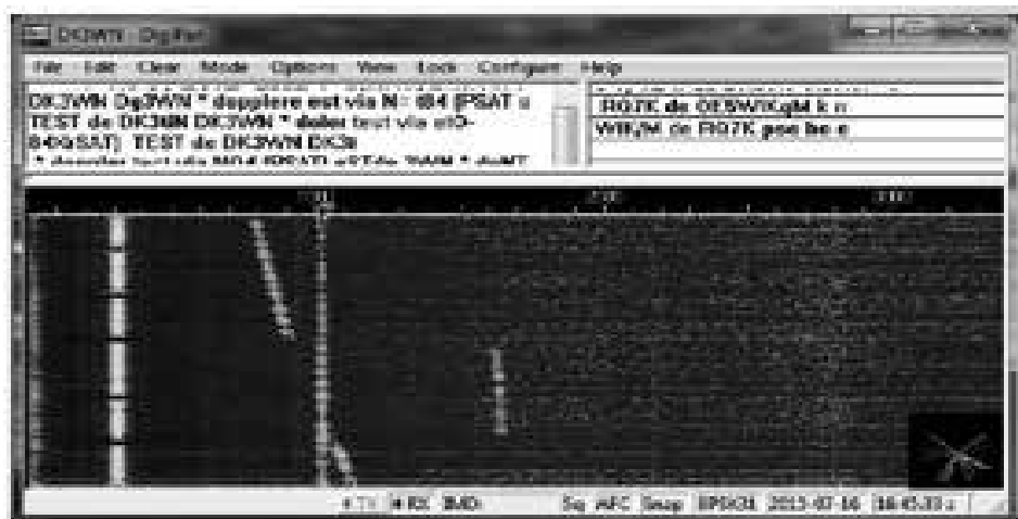
Figure 4 - Downlink waterfall shows stations with and without Doppler shift correction.
