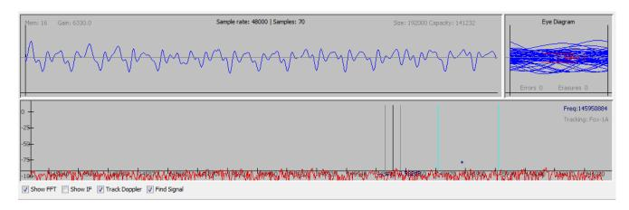
When FoxTelem finds a signal in the expected frequency range, it checks to see if it contains valid satellite telemetry. If it does, then it pauses the scan and decodes the data in the normal way. You should leave Track Doppler checked so that FoxTelem will follow the doppler on the satellite.
