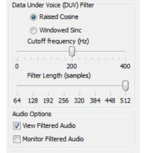
with other things, such as running experiments and taking photos, so the filtering on the spacecraft is very light (computationally). We therefore work a bit harder at the ground station and run a <u>Raised Cosine</u> filter or a <u>Windowed Sinc</u> filter.
