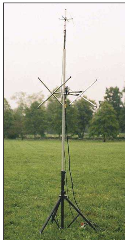
Figure 7 — The EZ-Lindenblad as a portable or Field Day antenna. A 70 cm antenna is on the top.
