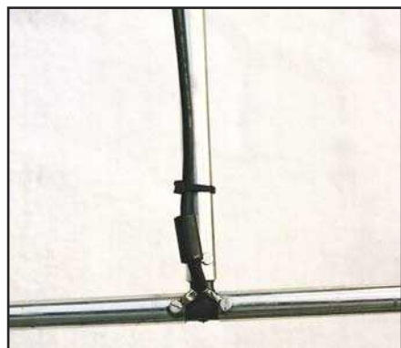
Figure 2 — Close-up of dipole electrical connections.
