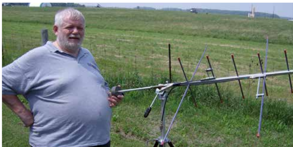
A number of AMSAT's experimenters have adapted the Arrow Antenna design to a wide range of unique tracking mounts. Here, Art VE3GNF shows off his "Gizmo" mount. The design features a small counterweight and "plumber's tee" that allows for a single movement (similar to an equatorial telescope mount) to track satellites across the sky.
