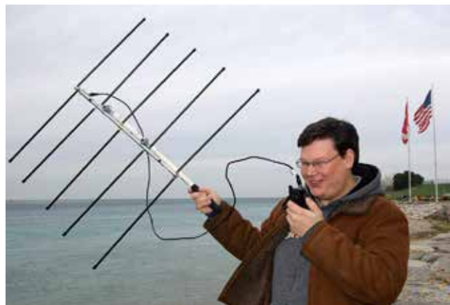
Another popular commercially made hand-held satellite antenna is the Elk. Here, Craig Wolsey, AC8EJ/VA3ICW, uses his HT and an Elk Model 2M/440L5 antenna to make a contact through one of the AMSAT satellites from the shores of Lake Huron in Canada. The antenna's unique log periodic design allows for dual band VHF/UHF operation using just five elements connected to a single feed line, all without the need for a duplexer.
