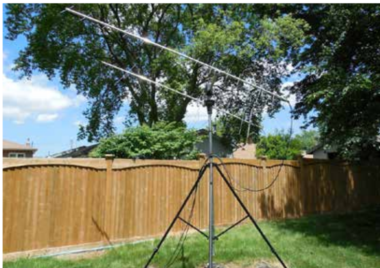
A portable satellite antenna array can also be used in a semi-permanent (or even permanent!) setup. My principle satellite antennas consist of an M2 Model 2MCP14 for 2m and a M2 436CP30 for 70cm. The array is mounted on a metal cross-boom with a Yaesu G-5400 rotator and an MFJ Model 1921 Heavy Duty tripod. Mounting the 2m antenna at a 45-degree angle on the cross boom helps to minimize interference to the circularly polarized pattern.
