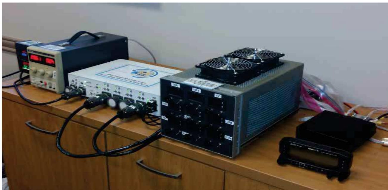
Figure 1 — The Kenwood D-710 GA radio is shown on the right side of the Interoperable Radio photo. Also, you can see the AMSAT-built power supply (in white) and the load simulators (to the right of the power supply) and power sources to the left of the power supply. [Courtesy of ARISS.]
