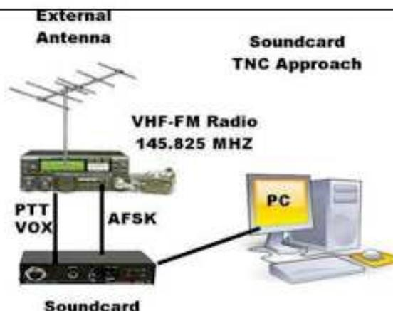
Figure 5 — Basic configuration of a soundcard-based packet system.
