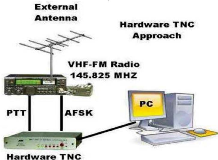
Figure 4 — Basic configuration of a hardware-based packet system.
