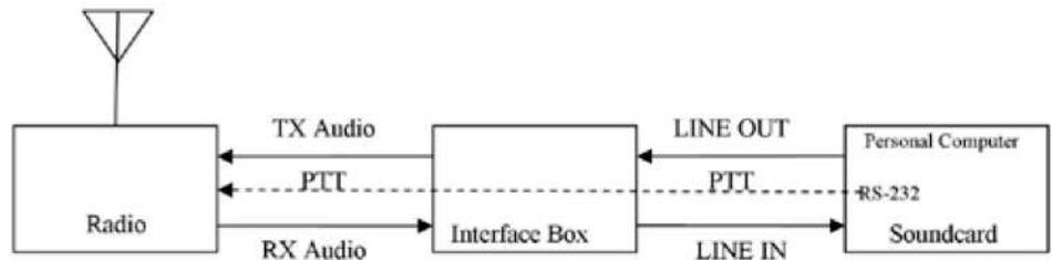
radio to the soundcard for other Amateur Radio applications such as RTTY, PSK31, JT65, and SSTV, you are already set for AX.25 ARISS packet operation with the ISS. All you need is to download, install, and configure some free software.
