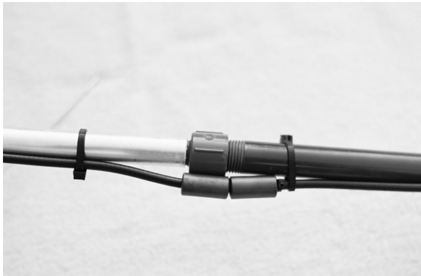
Figure 8. Ferrites aligned with bottom of driven dipole
