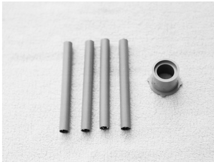
Figure 3. Standard PVC components used to make polarizer structure
