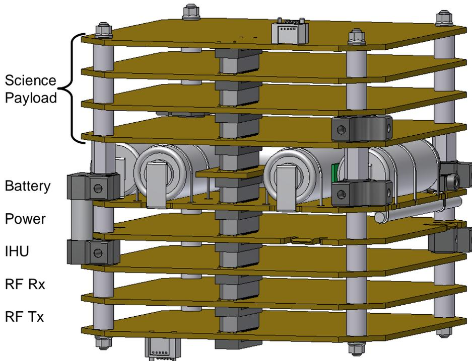
At the bottom of the stack is the RF Tx card which is the 2-meter transmitter. It will provide a minimum of 400mW output that will make the satellite very easy to hear. Next up is the RF Rx card that has a very sensitive 70cm receiver using a low-noise preamp and a surface-acoustic-wave filter to minimize interference. The Internal Housekeeping Unit or IHU card provides the brains
