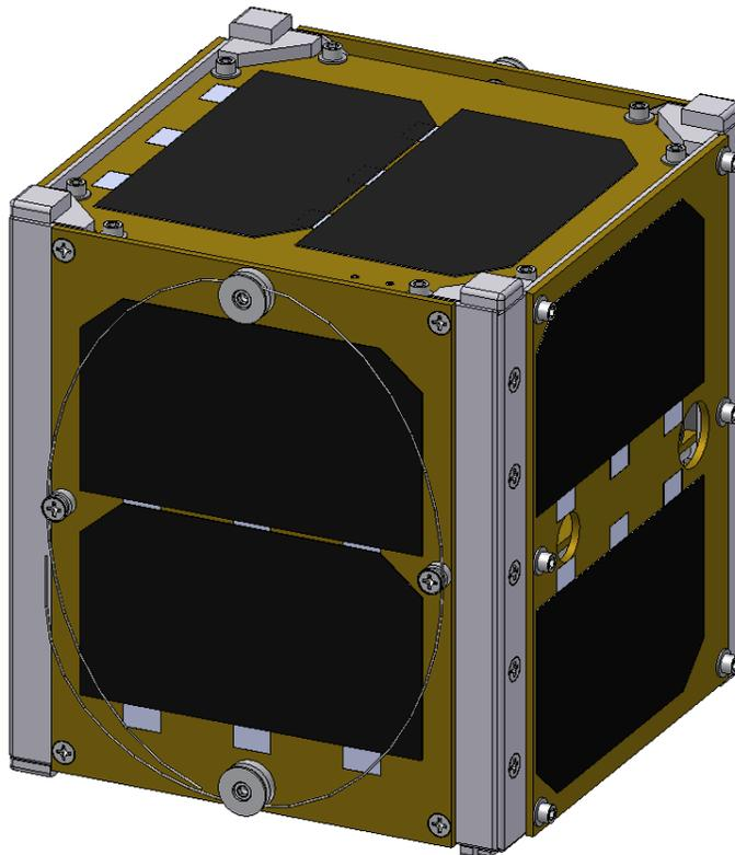
Each face of the satellite has a pair of high-performance, space-rated solar cells. These solar cells drive maximum-power-point-tracking, DC-to-DC converters that will wring out as much power as possible from the cells. This power is used to charge a 10 watt-hour NiCd battery. The power system can provide a little over 2 watts continuously, even in eclipse, and quite a bit more peak power if needed.
