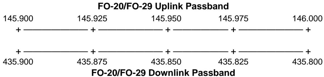
FO-29, launched in the fall of 1996, is virtually identical to FO-20 in regard to use of its analog transponder, even sharing the same passbands, so operation on this bird is no different than on its older sibling. Unlike FO-20, FO-29 is also active in the digital mode, with a packet BBS operating. Only one mode is available at one time, operating on a "round-robin" schedule, so don't expect the linear translator to be available at all times.
