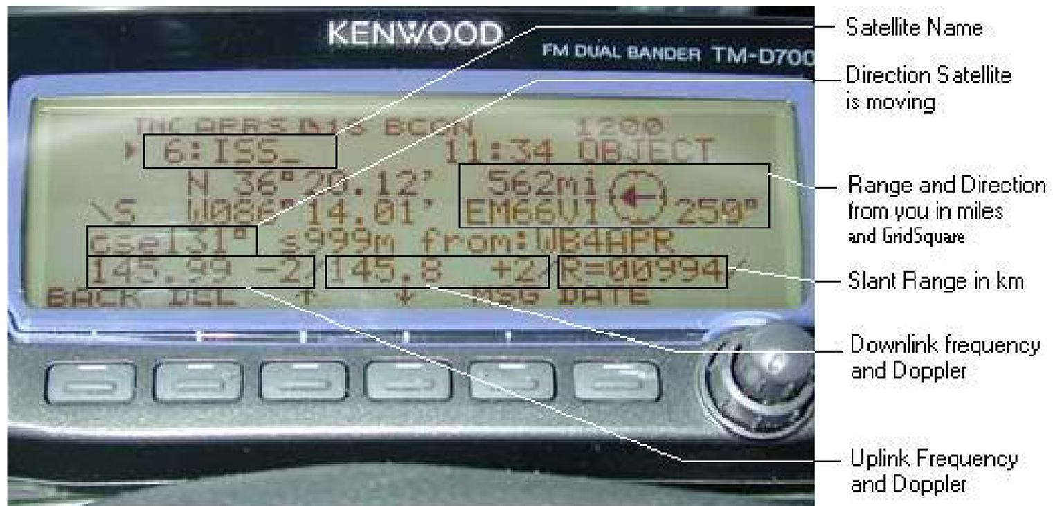
D-700 Front Panel Display of Satellite-in-view
