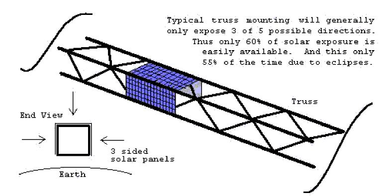
With about 1 square meter of solar cells on three panels the whole orbit average power available will only be about 12 watts. But low worldwide user demand duty cycles will permit peak payload demands of 80W over high user population areas.
