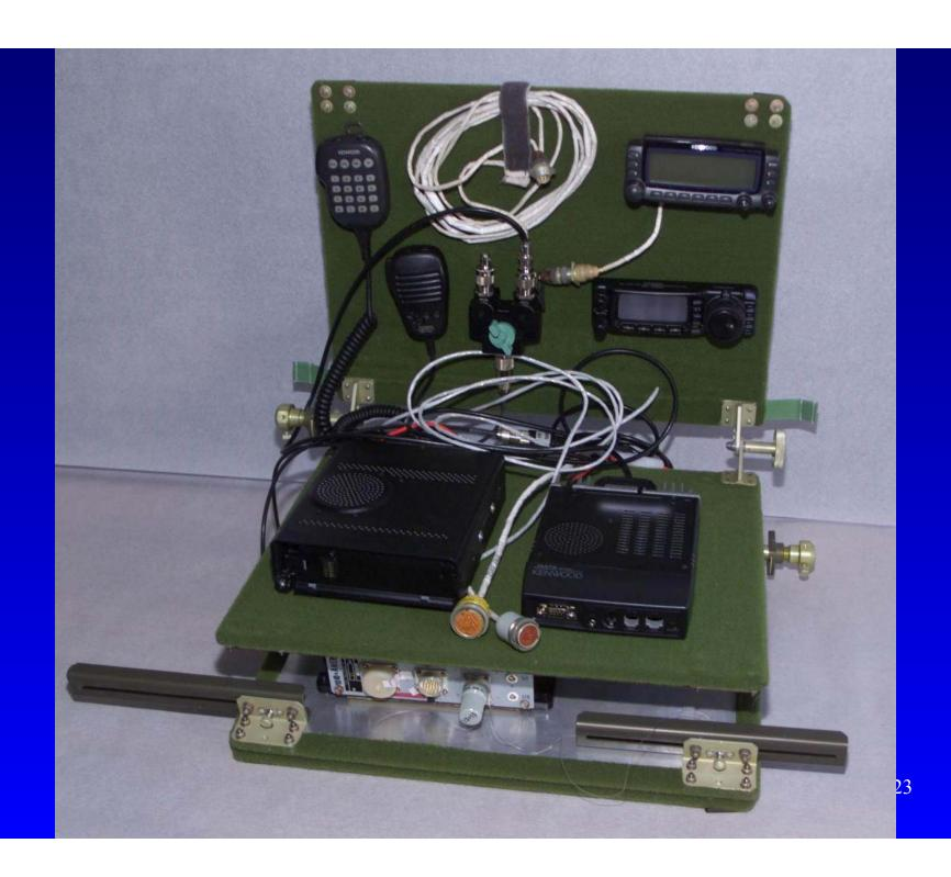
4 meter cable Length between Transceivers and microphones, control panels, & speakers
