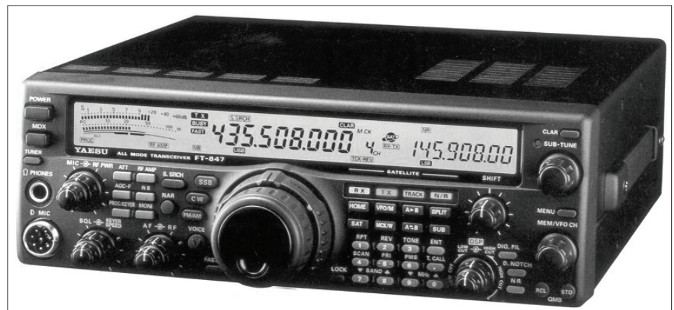
Figure 4: The Yaesu FT-847 is a 1990's-era, all-mode, HF/VHF/UHF base station radio that was specifically optimized for full duplex satellite work. While now out of production, it can sometimes still be found on the used market. (Courtesy: www.rigpix.com)
