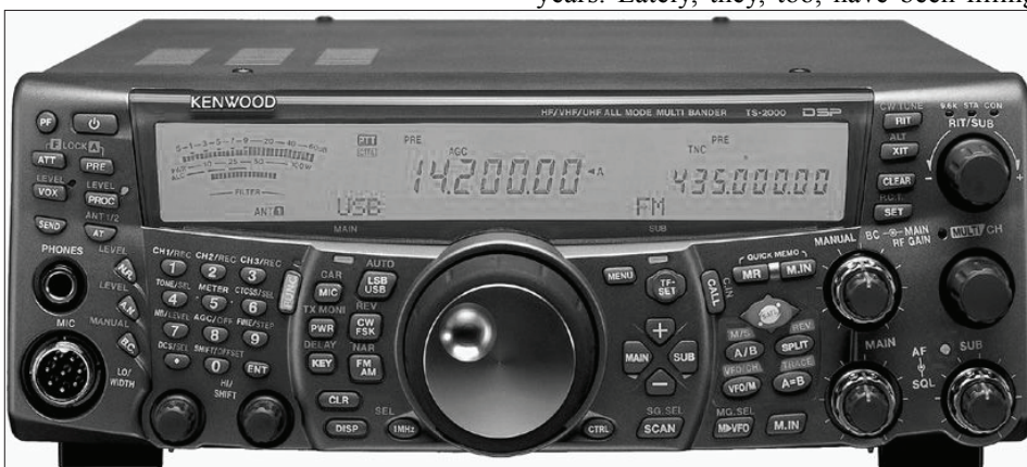
Figure 6: The Kenwood TS-2000 is another all mode HF/VHF/UHF base station radio suitable for full duplex satellite work that is, as of this writing, still in production. (Courtesy: Kenwood USA)
