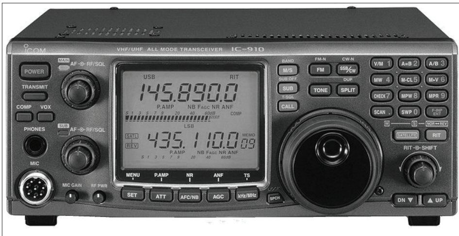
Figure 5: The ICOM IC-910H is a late model, all mode VHF/UHF base station that was specifically optimized for full duplex satellite work. This radio has recently been dropped from the ICOM lineup in favor of a newer satellite-capable model. However, start looking for the '910H to show up on the used market. (Courtesy: www.rigpix.com)
