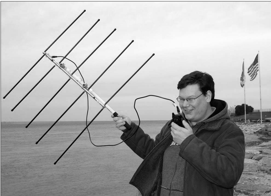
Craig Wolsey, AC8EJ/VA3ICW, uses his HT and Elk Model 2M/440L5 antenna to make a contact through AO-51 from the shores of Lake Huron in Canada. The antenna's unique log periodic design allows for dual band operation using just five elements connected to a single feedline and without the need for a duplexer.
