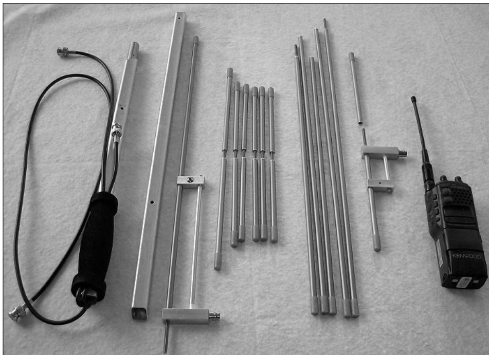
Photo 1: The author's satellite "hand shack" consists of an Arrow Model 146/437 antenna and a Kenwood TH-78A dual band handi-talkie (HT). The antenna easily breaks down into several pieces for easy transport. (KB1SF Photo)
