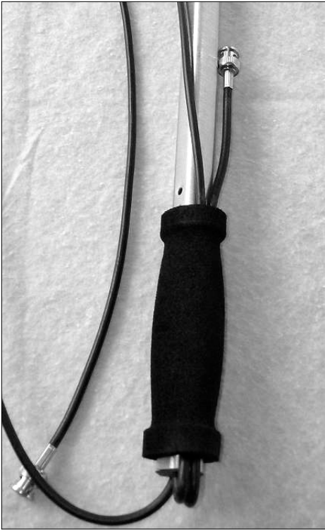
Photo 2: The Arrow sports a 10W 2m/70cm duplexer tucked inside the handle under a removable foam grip. This allows for a single feed line to connect the antenna to a “rubber duckie” connection on a handheld radio. (KB1SF Photo)
