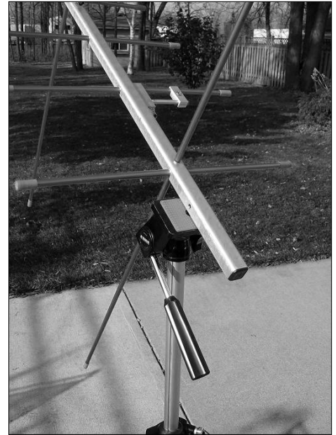
Photo 6: Removing the duplexer and foam grip reveals screw holes for mounting the Arrow Antenna on a lightweight photo tripod. (KB1SF Photo)
