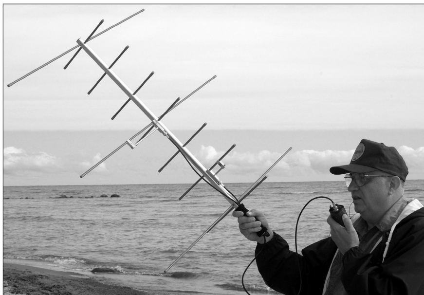
The author uses a Kenwood TH-78A dual-band HT and a lightweight Arrow Antenna to make a contact through AO-51 from the shores of Lake Huron in Michigan. When used with a 5 watt, full-duplex handheld in an open location free of foliage, such as a beach or a field, the antenna provides enough uplink and downlink gain to successfully work the FM birds, even on passes close to the horizon. (KB1OGF Photo)
