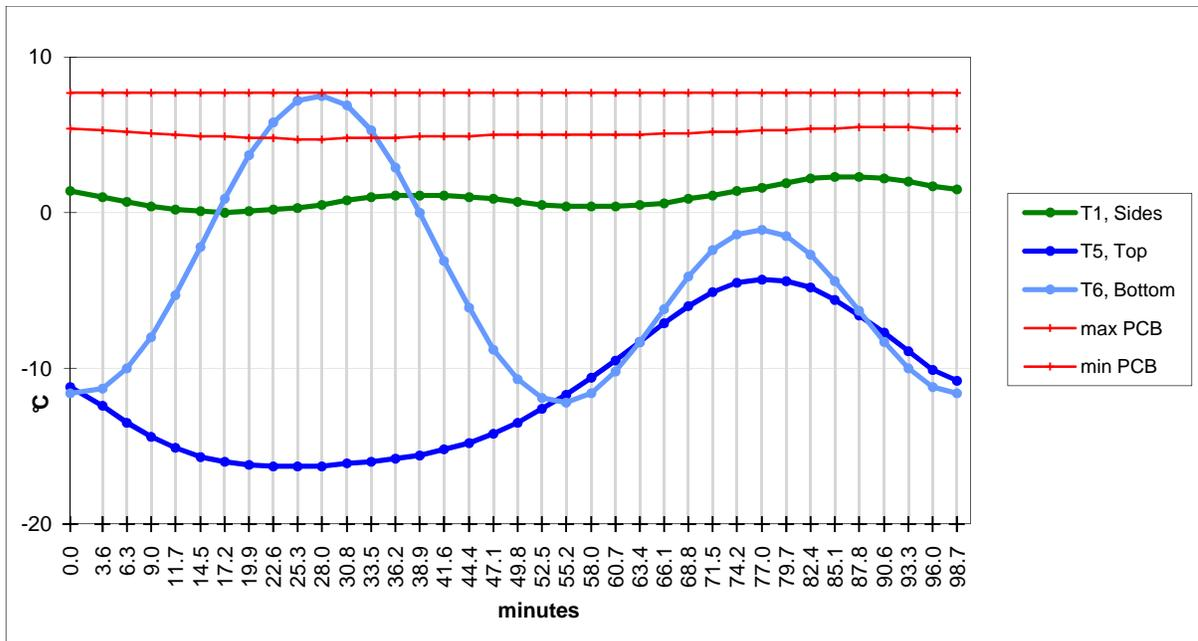
Fig 7 Fox-1 temperatures for full-sun orbit with thermally isolated electronics.
