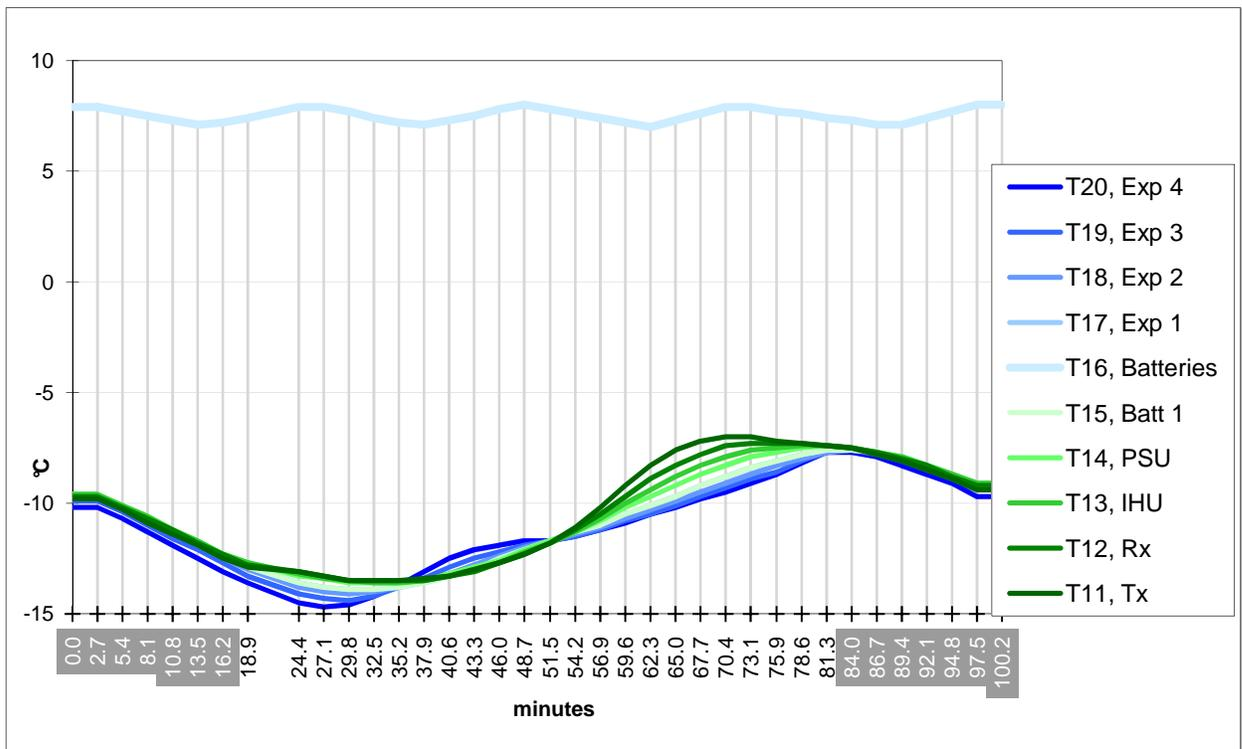
Figure 5 Fox-1 PCB temperatures for 33% eclipse orbit.
