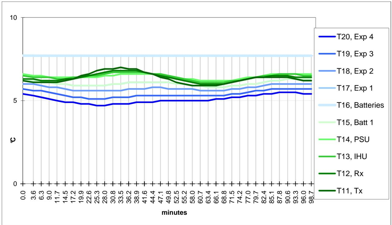
Figure 8 Fox-1 PCB Temperatures for full-sun orbit.
