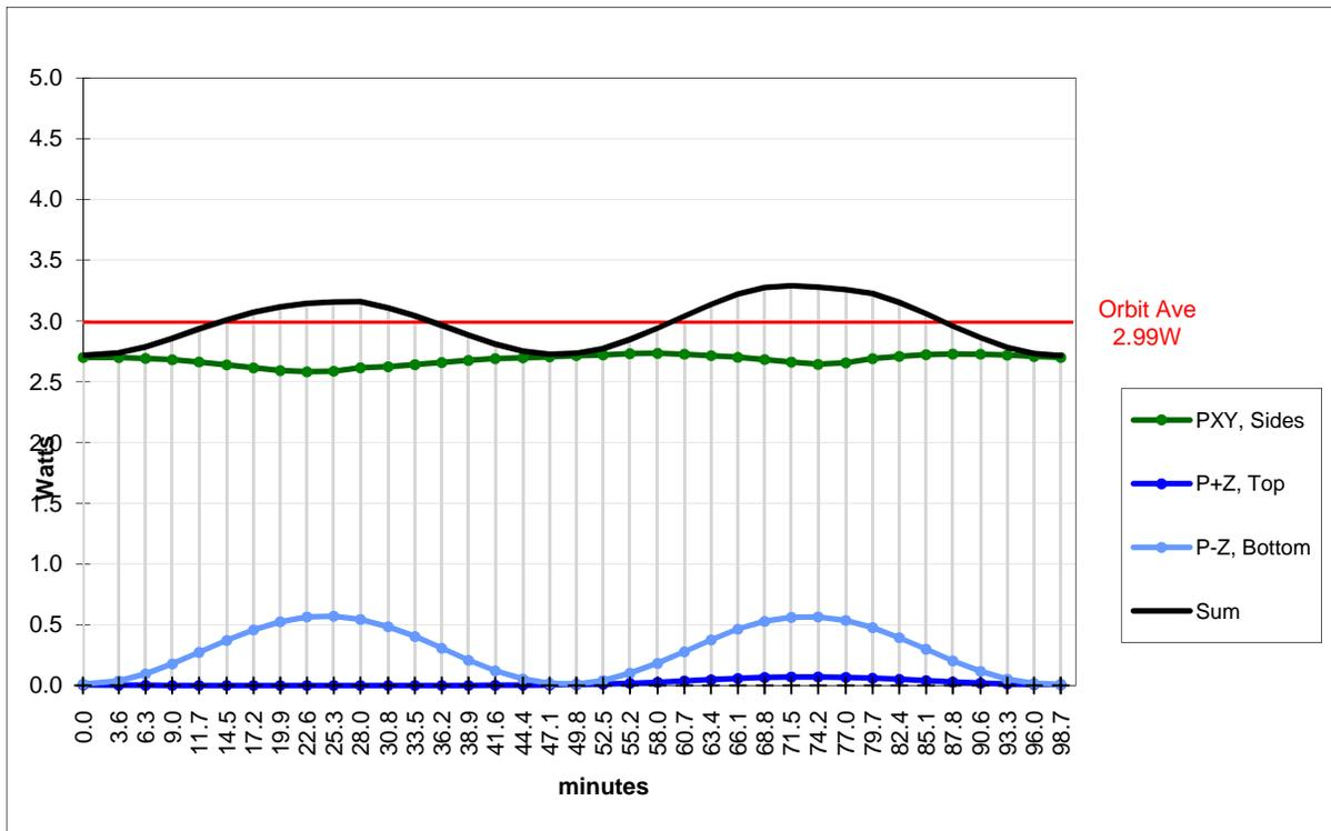
Figure 9 Fox-1 Solar power generation for full-sun orbit.
