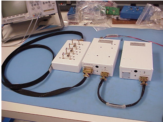
SuitSat Interface Control Box, Transmitter Box and Digitalker/Micro Controller Box Figure 4
