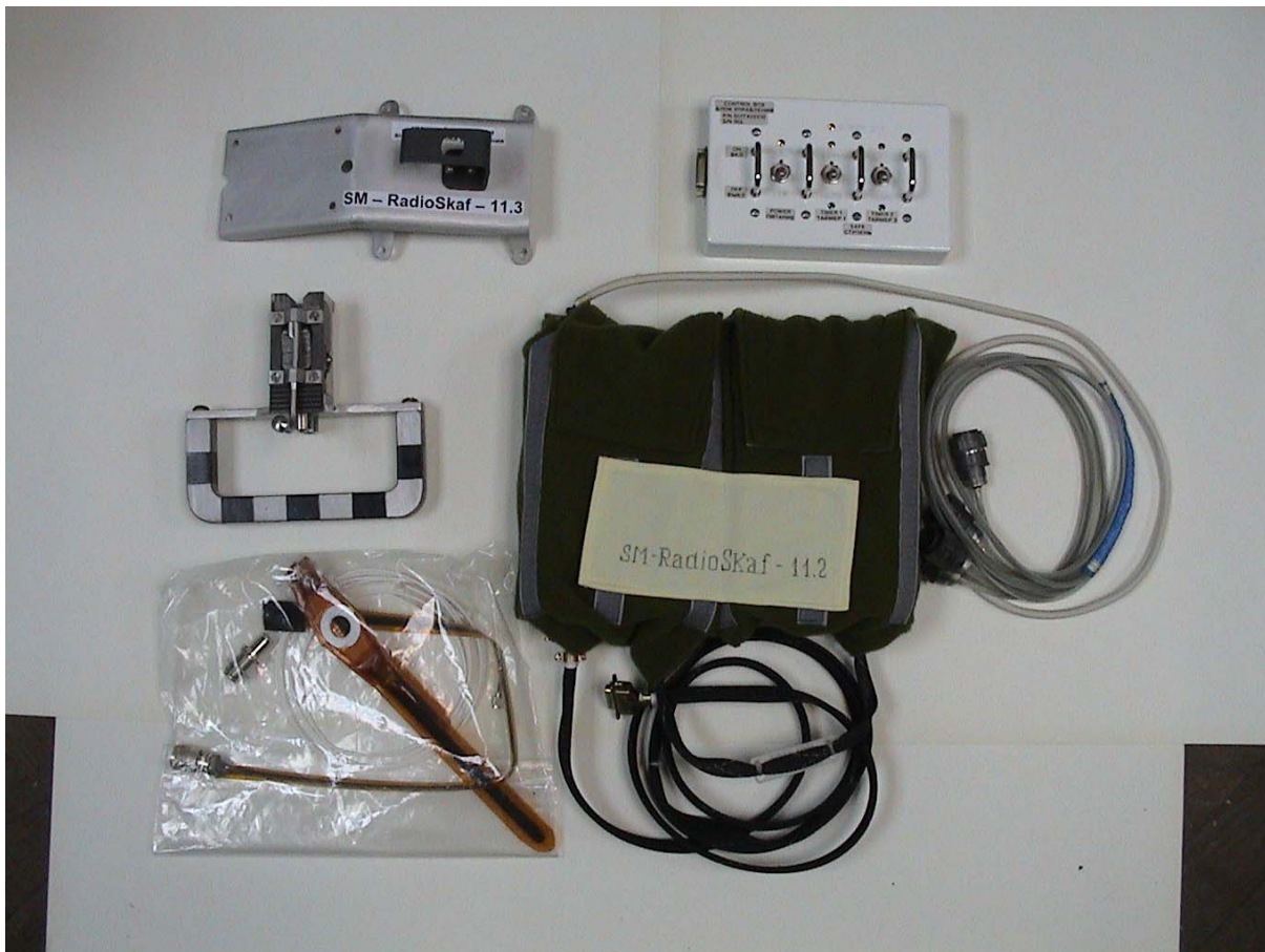
Suitsat Hardware -Transmitter and Digitalker/Microcontroller Box inside Fabric Container Figure 6
