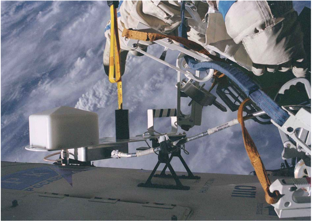
WA4 Antenna being Deployed During EVA Figure 10
