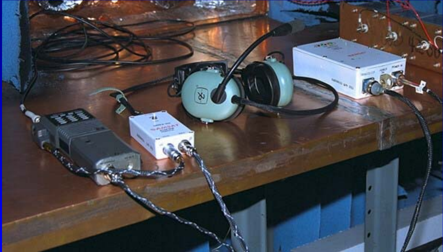
Initial Amateur Radio Station Undergoing EMI Tests at GSFC
