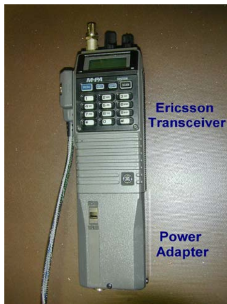
Transceiver & Power Adapter Figure 6
