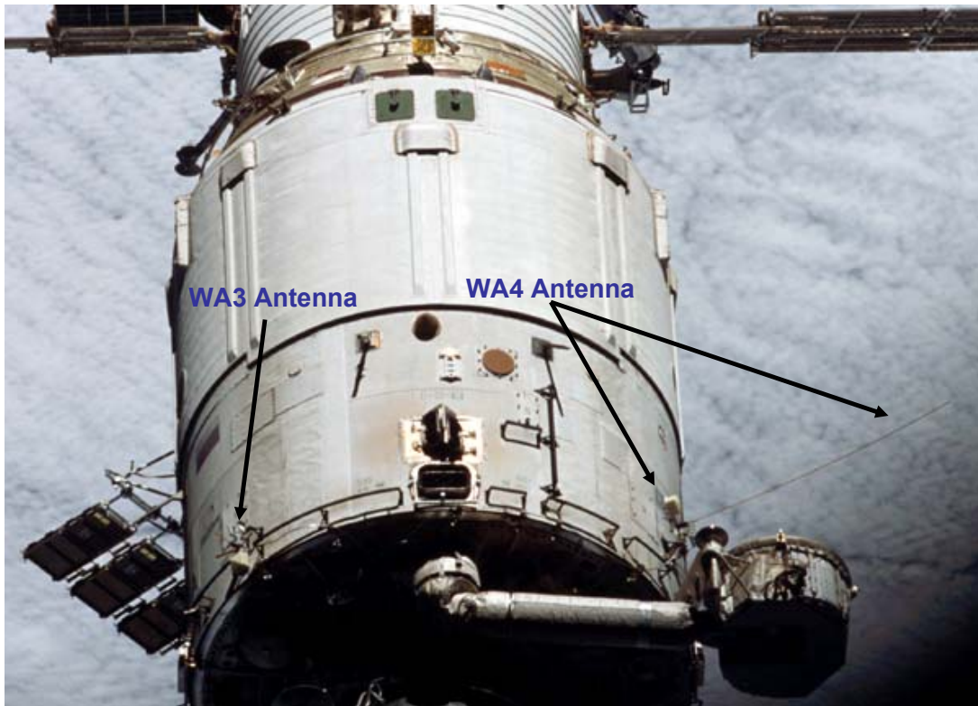
Zenith Mounted Antennas on Service Module Figure 15
