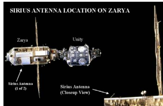
FGB 2 Meter Antenna Locations Figure 1
