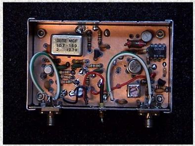
Amplifier and gain control of in-band signals
